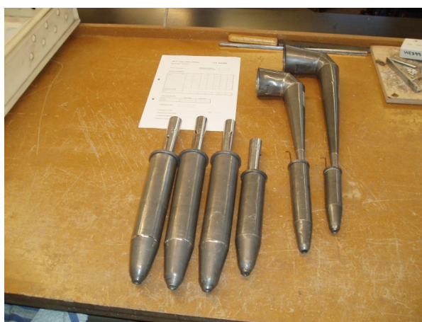
Tuba pipes and parts of the Pedal Ophicleide in the workshop in Durham
