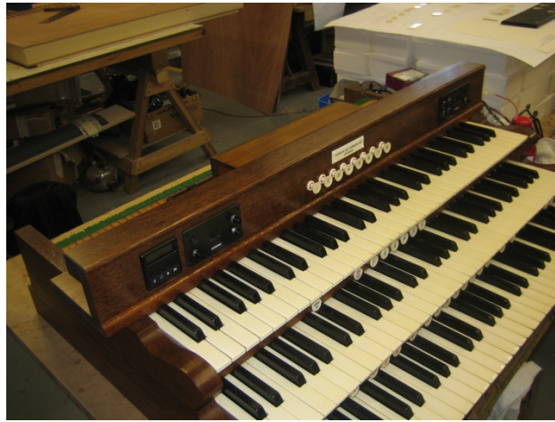
Three of the four keyboards in the workshop at Durham showing the pistons and the new fascia control panels
