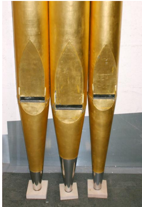
Another view of the repaired front pipes, before re-gilding, showing the new pipe tips
