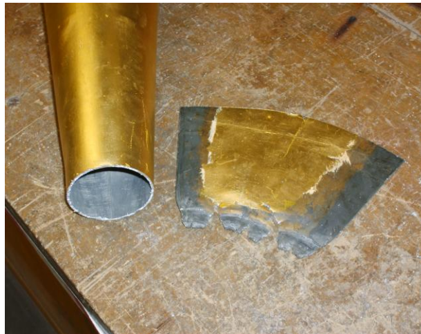
A pipe tip removed and flattened. The shape can now be used to prepare a new tip in pipe metal
