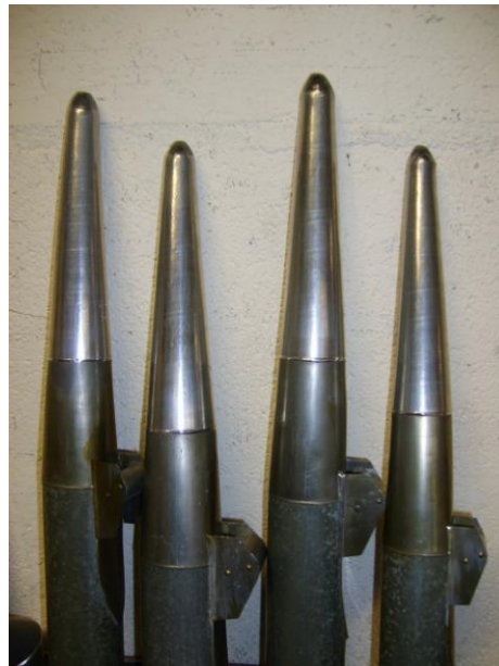
New tips for pipes of the Violes stop
