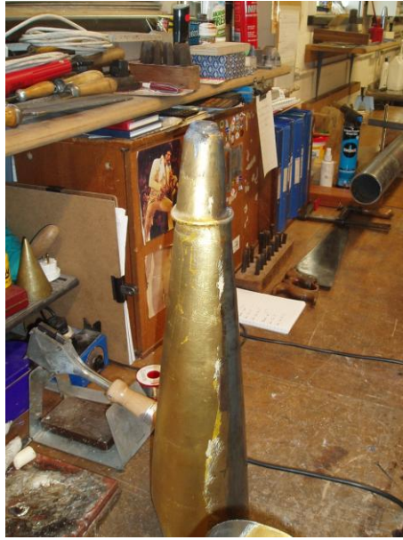
The damaged tip of a pipe foot
