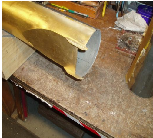
Pipe body with foot removed. Note that the pipe ears are still in place
