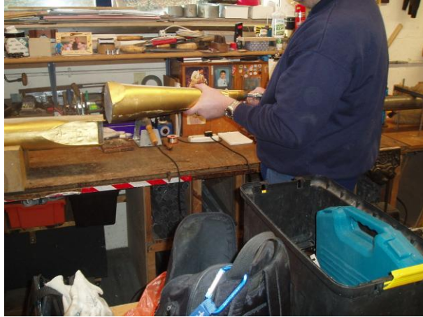
A foot has just been removed from a front pipe
